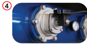
MEMBRANE ELECTRO VALVE: two way valve normally closed; it is activated by an electric solenoid. It holds air pressure of max.7 bar. The compressed air tank operates at 4 to 7 bar.
