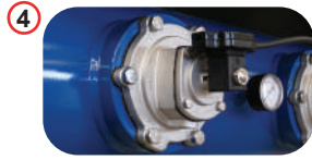
MEMBRANE ELECTRO VALVE: two way valve normally closed; it is activated by an electric solenoid. It holds air pressure of max.6 bar. The compressed air tank operates at 4 to 6 bar.
