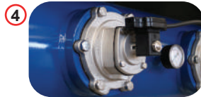
4 MEMBRANE ELECTRO VALVE: two way valve normally closed; it is activated by an electric solenoid. It holds air pressure of max.6 bar. The compressed air tank operates at 4 to 6 bar.
